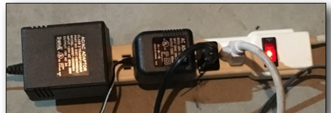
(A6) Power supply with protective device. The Digitrax Zephyr has a built-in circuit breaker protection plus each block has the 1156 tail light bulbs as shown in A1. Additionally, the power supplies are plugged into a surge protector power strip.
