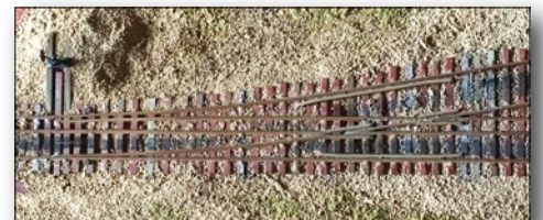
(B6) Gauge Separation Turnout
